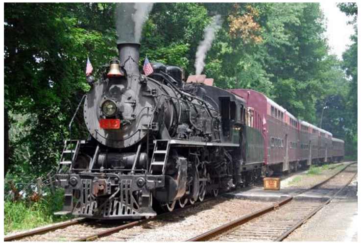
NYS&W #142, a 2-8-2 "Mikado-Type" steam locomotive, powers the NYS&WT&HS's "Mine Train" train ride at Phillipsburg, NJ on July 9, 2010. (Photo by Ed Kaminski)
