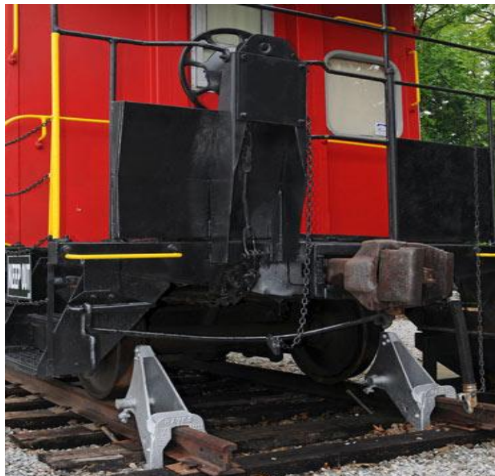
In the spring of 2011, MSHC member Vince Molodowec carefully restored two original "S-Type" Hayes track bumpers that were once found on the Maywood Station team track siding installed them at the end of the panel track beneath Maywood Station Caboose 24542. This view of Vince's completed project was taken on May 15, 2011. (Photo by Robert P. Pisani)
