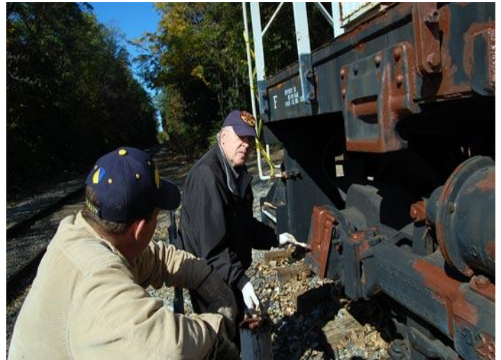
MSHC members Mike Szymanski and Joseph Katzenstein work on cleaning up and priming NYS&W #206's underframe on October 19, 2008. (Photo by Ed. Kaminski)
